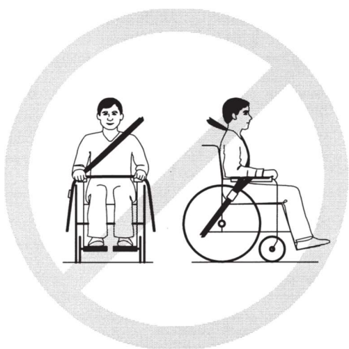
Fig 20.5.D Improper adjustment of belt
